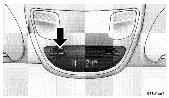
Use this button to reset the following displays: Average Fuel Economy (AVG ECO) Trip Odometer (ODO) Elapsed time (ET)
